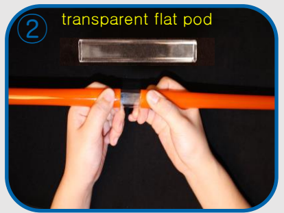
2 Insert two 60cm frames into a transparent flat pod frame. Create 80 identical units.
