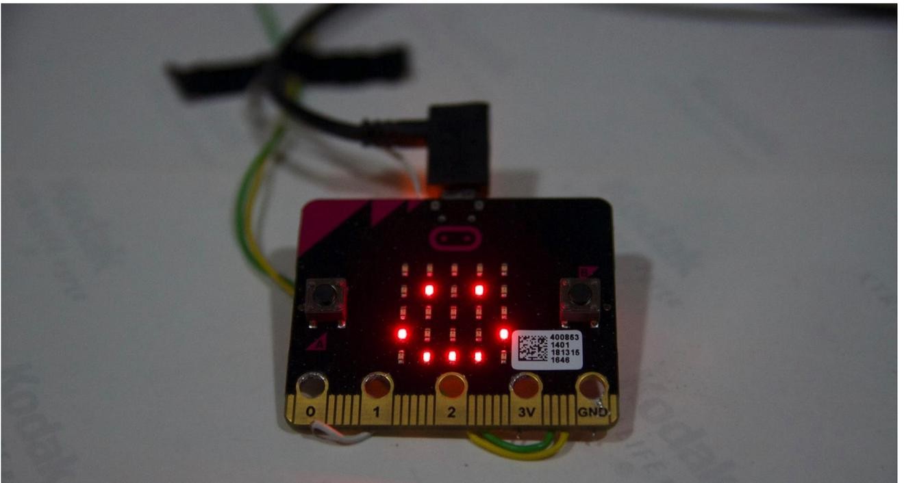
Testing the micro:bit at home is easy because the board can be programmed via a webpage.
